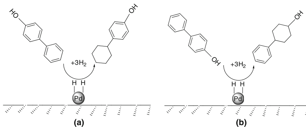
Scheme 1 Proposed adsorption modes of p -PP over different supports. a Adsorption of benzene ring in p -PP firstly and gives rise to p -CP. b Adsorption of phenol ring in p -PP firstly and gives rise to p -PC
